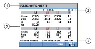
This screen gives a quick overview of important numerical measuring values. An example is the table belonging to VOLTS/AMPS/HERTZ mode.
