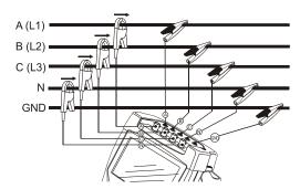
Figure 1. Connection of Analyzer to 3-phase distribution system
