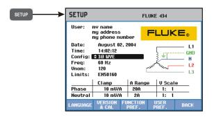
The SETUP key gives access to a menu to configure the Analyzer for your measurements.
