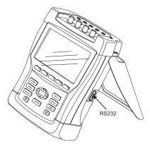
The Analyzer has a tilt stand that allows viewing the screen at an angle when placed on a flat surface. With the tilt stand folded out, the optical port at the right side of the Analyzer can be accessed.
