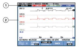
The Trend screen shows the changes over time of measuring values on one row of the table. An example is the VOLTS/AMPS/HERTZ TREND. Time is displayed horizontally. The display is built up from the right side of the screen. To allow continuous recording of data, the time axis is compressed when necessary.
