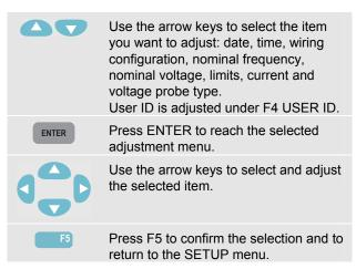
Note: Limits gives access to submenus to recall, customize, and save 6 sets of Power Quality criteria. For detailed information refer to *Chapter 18 in the Users Manual* on the accompanying CD-ROM.
